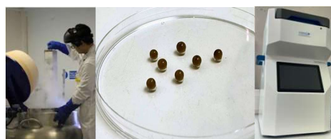
Fig 5. (L to R) Cryotank, Encapsulated soil in calcium alginate beads before storage in liquid nitrogen and the ViaFreeze Duo Controlled rate cooler
